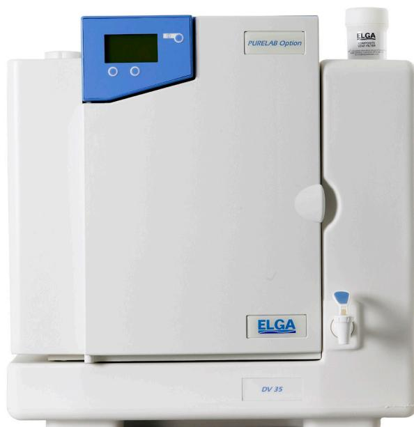
**PURELAB Option-R 7/15.** This system provides pure water on demand with a range of flow-rates suitable for many general molecular genetics applications.
